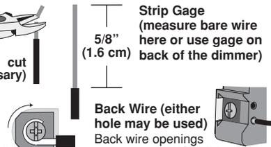
Strip Gage (measure bare wire here or use gage on back of the dimmer)
