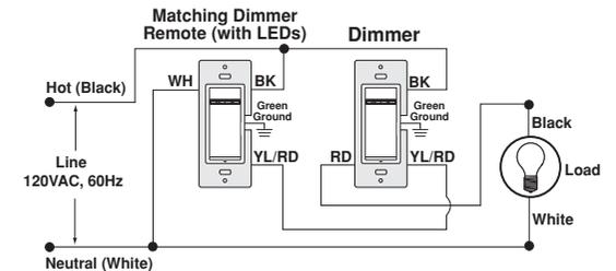
**NOTE:** The dimmer must be installed in a wall box that has a Load connection. The matching remote must be installed in a wall box with a Line Hot connection and a Neutral connection. A Neutral wire to the matching remote needs to be added as shown. If you are unsure about any part of these instructions, consult a qualified electrician.
