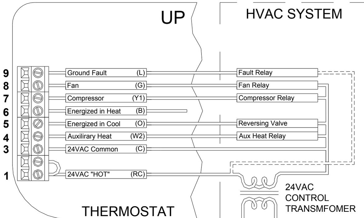
**Figure 7 – Connections for heat pump thermostat**
