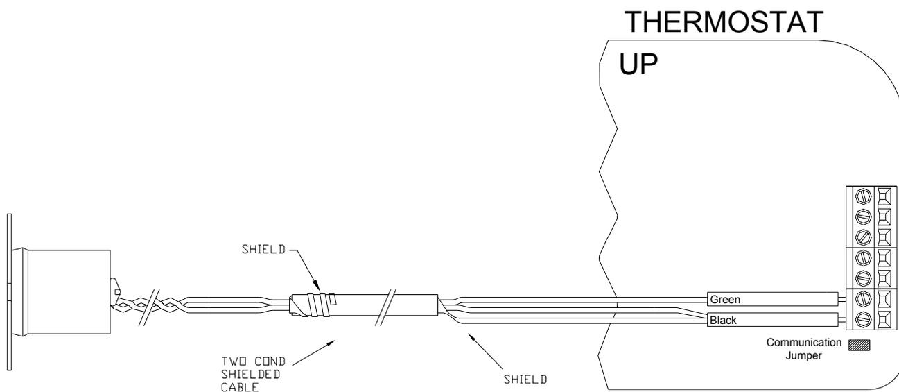
**Figure 11** – *Connections to a Remote Temperature Sensor*
