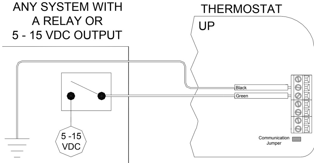
**Figure 10** – *Connections to a Remote Setback Switch*
